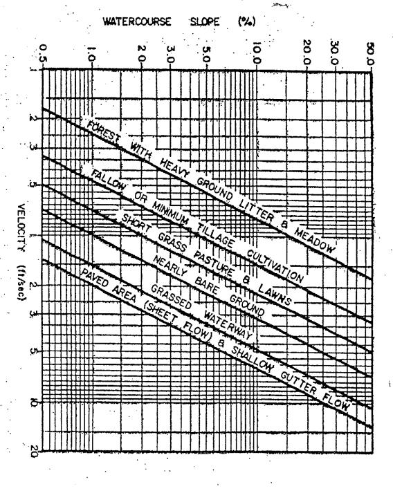
The average velocities for estimating travel time for overland flow (SCS method). (Source: SCS, 1975.)
